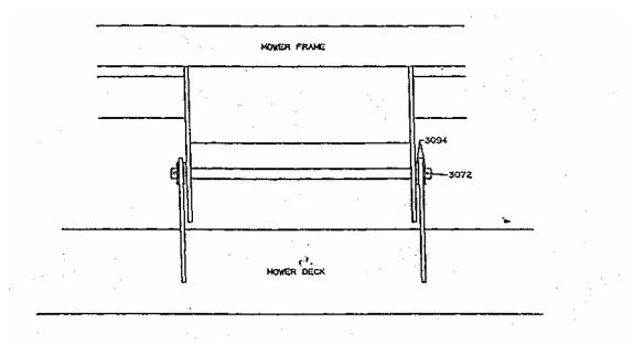
2. Attach short L-rod (P/N 1355) to lift arms as shown in drawing.
